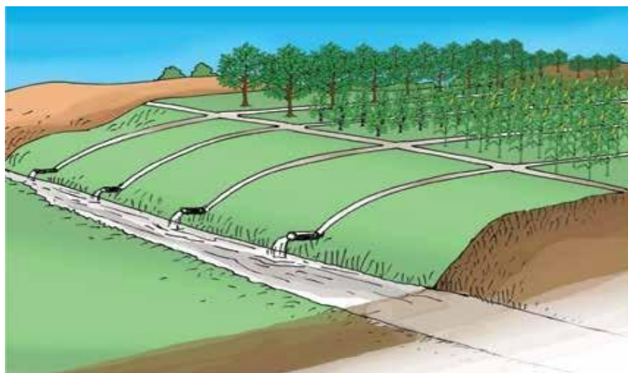
Figure 6.21 Drainage Channel (Source: Godinho et al. , 2023)
